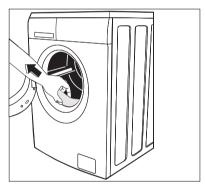
**8.** Fill the smaller upper hole and the two large ones with the corresponding plastic plug caps supplied in the bag containing the instruction booklet.
